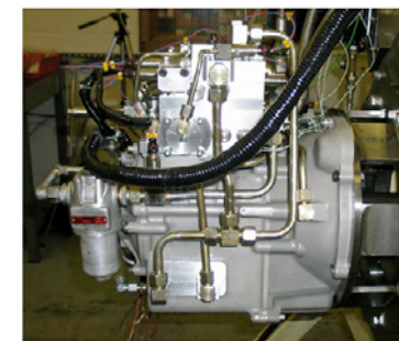
Prototype C-IVT - Under test at Torotrak
