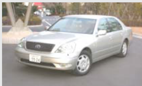
Lexus LS430 SHTV – IVT fitted to a Lexus by NSK
