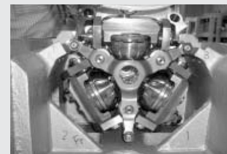
Assembled power rollers in one cavity
