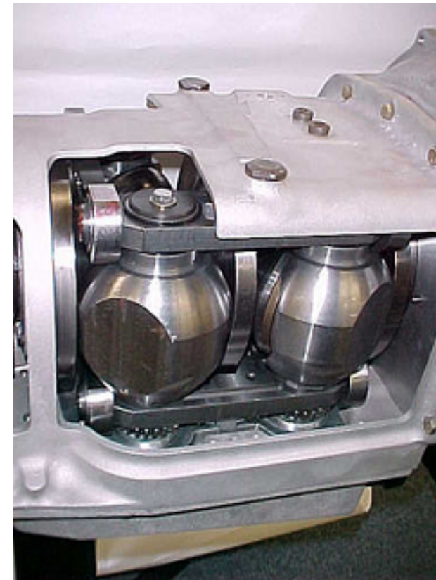
Cut-away view of a continuously variable transmission (CVT) under development at Transmission Technologies Corporation.
